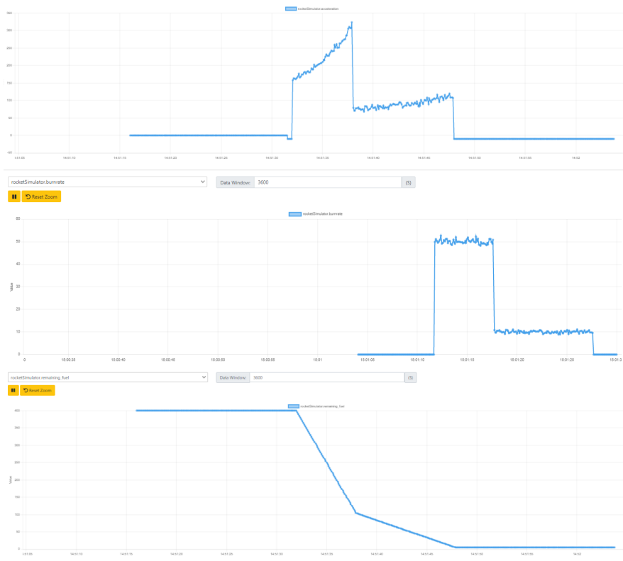
Figure 8: Some values of the rocket plotted (acceleration, burnrate, remaining fuel) over time)
